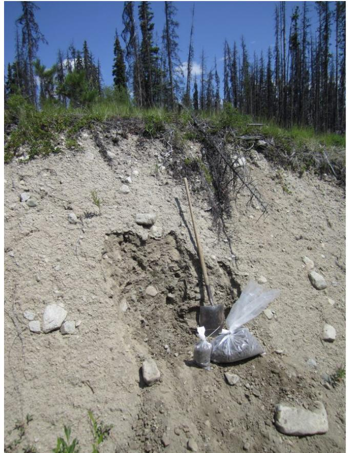
**Fig. 9.** Typical subglacial till sample site (15PMA053) with large (9 to 15 kg) and small (1 to 2 kg) samples. View is towards north. Shovel is 1.6 m long.
