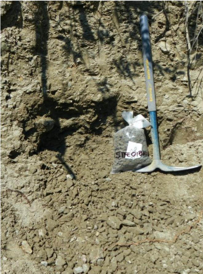
**Fig. 6.** Well-compacted, matrix-supported, fissile, diamicton, with clasts (about 15%) floating in a predominantly sandy silt to silty sand matrix that also contains about 6% clay. Interpreted as subglacial till. This site (15TFE018A01) is 6 km west-northwest of the Valley deposit. Pick is 62 cm long.
