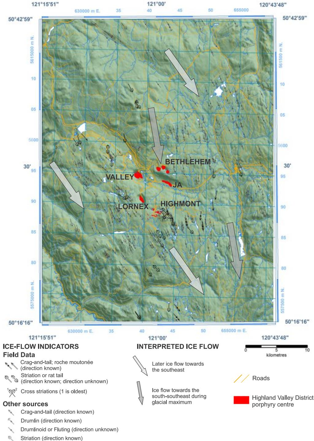
**Fig. 4.** Ice-flow indicators of Highland Valley Copper mine area. Interpreted ice-flow directions are generalized from data points shown, taking into account topography and expected thickness of Cordilleran ice sheet during full-glacial and late-glacial conditions. Field data from Plouffe and Ferbey (2015a), other sources from Ferbey et al. (2013).
