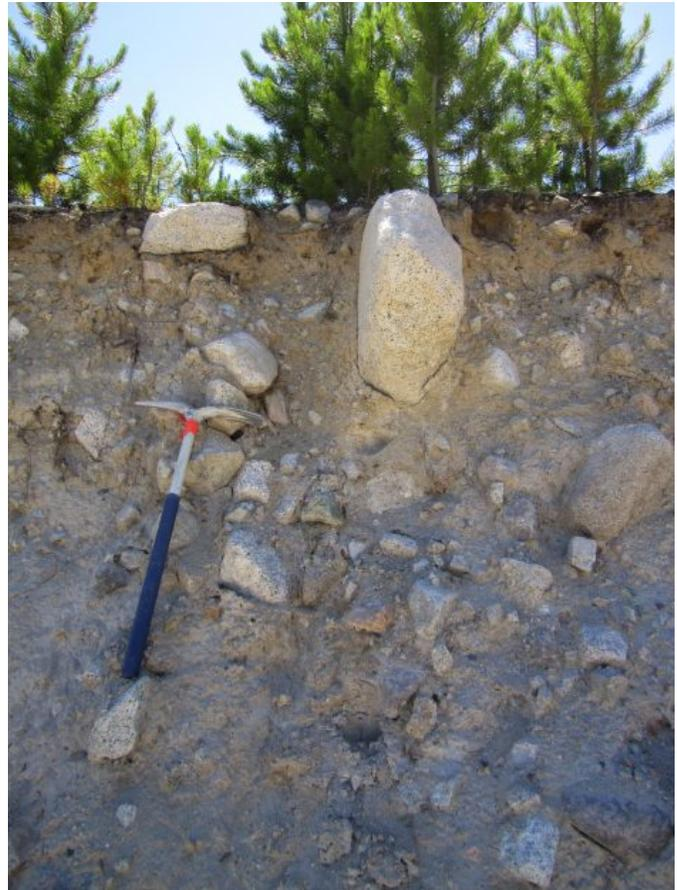
**Fig. 7.** Poorly compacted, massive, bouldery diamicton, with clasts (about 35%) floating in a predominantly silty sand to sandy silt matrix with about 2% clay. Near-vertical boulder suggests deposition by meltout. Interpreted as ablation till. Site (15PMA108A01) is 7 km south of the Highmont deposit. Pick is 62 cm long.
