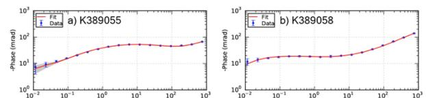
**Figure 3. Phase spectra and fit with the Debye decomposition approach for rock samples (a) K389055, and (b) K389058. Both phase curves display the high-frequency response ( $> 100$  Hz) associated with processes unrelated to the electrical double-layer. Sample K389055 has a phase peak of -53 mrad at a frequency of 5.86 Hz and sample K389058 has a phase peak of -19 mrad at 0.37 Hz. The optimal parameters produce a response that fits the data within the measurement uncertainty in both cases.**
