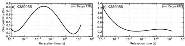
**Figure 4.** The complex resistivity spectra of samples K389055 and K389058 are fitted with a 4<sup>th</sup> and 3<sup>rd</sup> order polynomial Debye relaxation time distribution (RTD), respectively. The first sample has a maximum chargeability of 0.81% at a peak relaxation time of 0.02 second. The second sample has a maximum chargeability of 0.33% at a peak relaxation time of 2 seconds, when not considering the high-frequency response.
