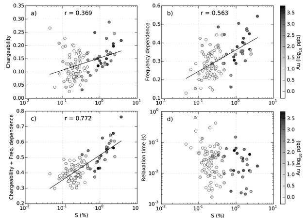
**Figure 6.** Correlations between sulphur content and Cole-Cole chargeability (a), frequency dependence (b), and the addition of both parameters (c). The relaxation time parameter does not appear related to the total sulphur content (d). Only meta-sedimentary rocks of the Canadian Malartic gold deposit are considered.
