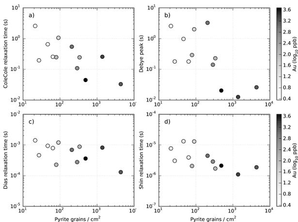
**Figure 5.** Relaxation times obtained by stochastic inversion on 12 rock samples from the Canadian Malartic gold deposit. The greyscale legend bar indicates the gold content of each sample. In the Cole-Cole model (a), rock samples with over 1000 ppb Au tend to possess a characteristic relaxation time that is lower than 0.1 second. The same observation is made when using the Debye decomposition approach and considering the peak relaxation time (b).
