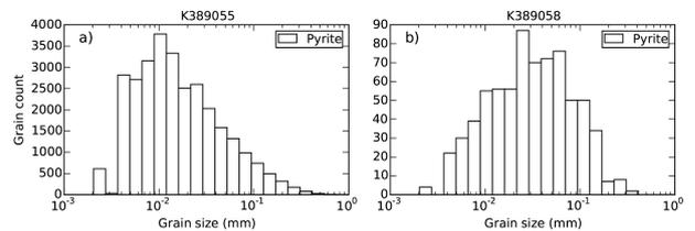
**Figure 2. Grain size distribution of pyrite, the main sulphide mineral in samples K389055 (a) and K389058 (b). The first sample has a median pyrite grain size of 14 microns, and contains up to 1330 ppb Au and 3.57% pyrite. The second sample has a median grain size of 30 microns, and contains up to 34 ppb Au and 0.19% pyrite.**
