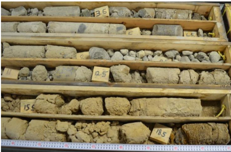
Figure 4 Photo of the transition from Sm (massive sand) lithofacies unit to Dmm (matrix-supported, massive diamicton) and Bcm (clast-supported, massive boulders) units of core VTH2014-03, at a depth of 0-18.7m. Lithofacies code from Evans and Benn (2004).
