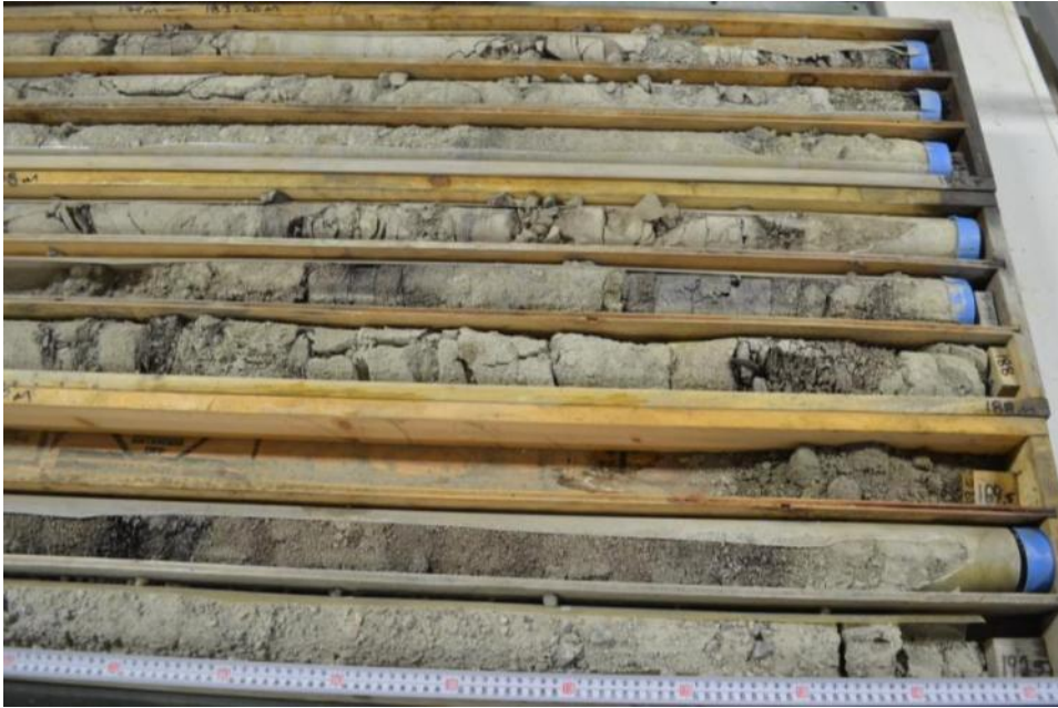
Figure 5a Photo of the alternating Sm (massive sand) and Fm (massive silts and clays) lithofacies units of core VTH2014-06, at a depth of 179.0-192.5m. Lithofacies code from Evans and Benn (2004).
