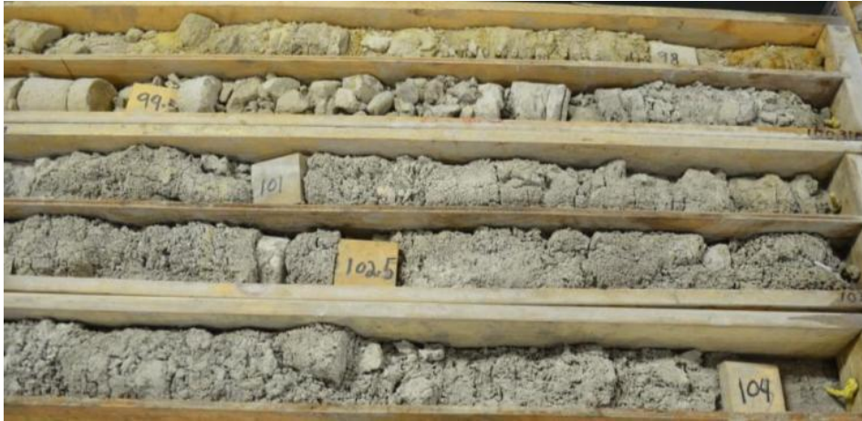
Figure 2a Photo of the thick FI (finely laminated silts and clays) lithofacies unit of core VTH2014-03, at a depth of 96.9-104.0m. Lithofacies code from Evans and Benn (2004).
