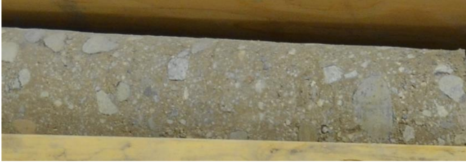
Figure 11b A close-up image of one of the Dmm (matrix-supported, massive diamicton) units from drillcore VTH 2014-09. Note the angularity of the framework clasts, the silty texture of the matrix and the stiffness.
