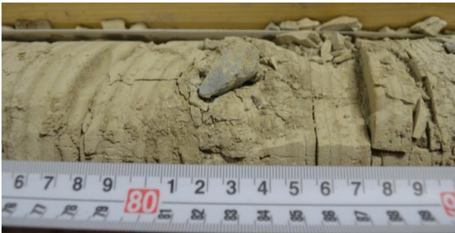
Figure 5b Photo of an SI (sand with horizontal and draped laminations) lithofacies unit and rounded pebble of core VTH2014-06, at a depth of 73.3m. Lithofacies code from Evans and Benn (2004).
