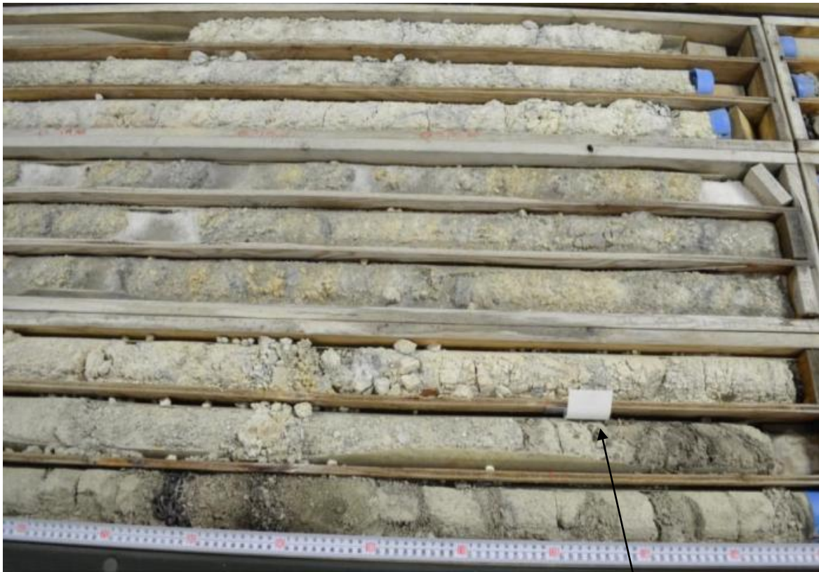
Beginning of coal lenses down core (core segment order right and down in photo)
