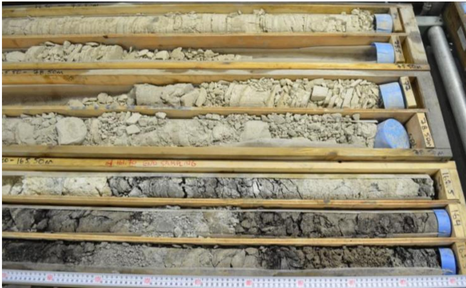
Figure 6 Photo of an SI (sand with horizontal and draped laminations) lithofacies unit and coal lenses of core VTH2014-06, at a depth of 72.5-165.5m. Lithofacies code from Evans and Benn (2004).
