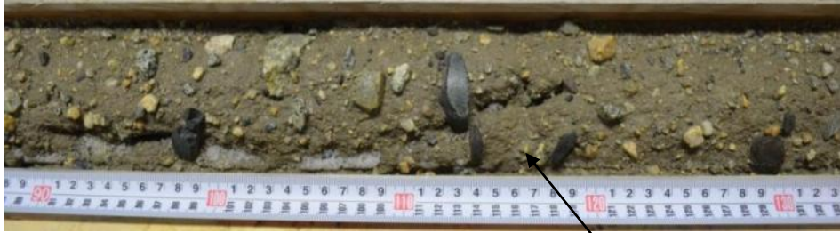
Figure 13 Photo of preferentially oriented clasts in one of the upper Dmm (matrix-supported, massive diamicton) lithofacies units of core VTH2014-09, at a depth of 51.9-52.3m. Lithofacies code from Evans and Benn (2004).
