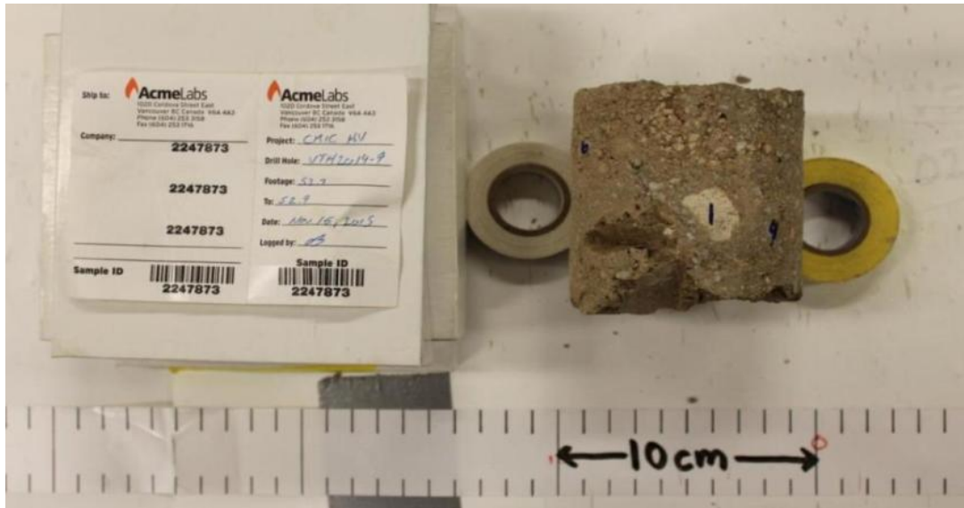
Figure 17 Taking magnetic susceptibility measurements across one of the samples.
