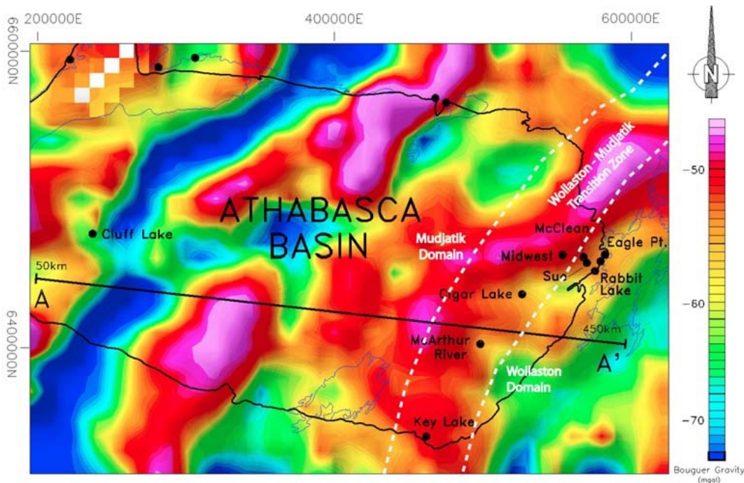
Figure 3.31: Corrected Bouguer gravity anomaly map for the Athabasca Basin. Black line shows the limit of Athabasca Basin (Matthews et al., 1997).
