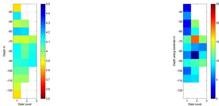
**Figure 4.8:** Apparent resistivity (left) and chargeability (right) pseudo-section along BR1 (Schlumberger array). Resistivity is in  $\log_{10}(\Omega m)$ . Chargeability is in  $mV/V$ . Electrode spacing is 8m
