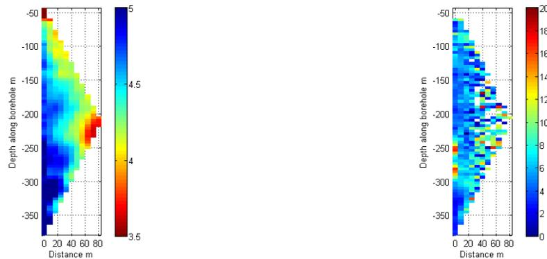
**Figure 3.8:** Apparent resistivity (left) and chargeability (right) pseudo-sections along borehole NRS130075 (Schlumberger array). Resistivity is in  $\log_{10}(\Omega m)$ . Chargeability is in  $mV/V$ . Electrode spacing is 4m
