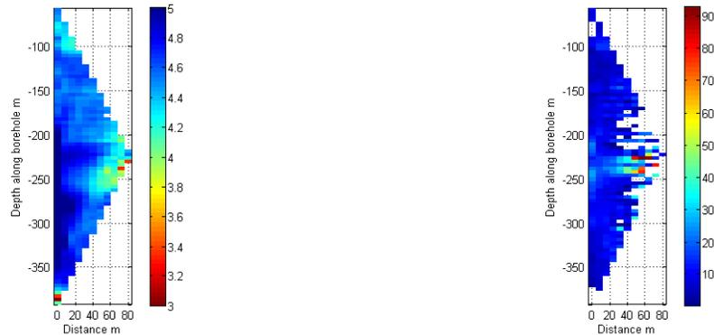
**Figure 3.2:** (Apparent resistivity (left) and chargeability (right) pseudo-section along borehole W121 (Schlumberger array). Resistivity is in  $\log_{10}(\Omega m)$ . Chargeability is in  $mV/V$ . Electrode spacing is 4m
