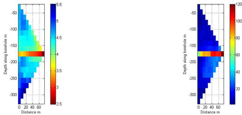
**Figure 3.11:** Apparent resistivity (left) and chargeability (right) pseudo-sections along borehole NRS170162 (Schlumberger array). Resistivity is in  $\log_{10}(\Omega m)$ . Chargeability is in  $mV/V$ . Electrode spacing is 16m
