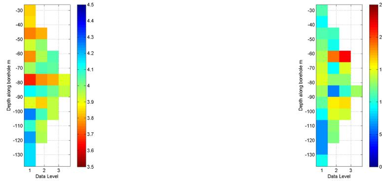
**Figure 4.9:** Apparent resistivity (left) and chargeability (right) pseudo-section along BR2 (Schlumberger array). Resistivity is in  $\log_{10}(\Omega m)$ . Chargeability is in  $mV/V$ . Electrode spacing is 8m
