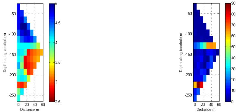
**Figure 3.10:** Apparent resistivity (left) and chargeability (right) pseudo-sections along borehole NRS170100 (Schlumberger array). Resistivity is in  $\log_{10}(\Omega m)$ . Chargeability is in  $mV/V$ . Electrode spacing is 16m
