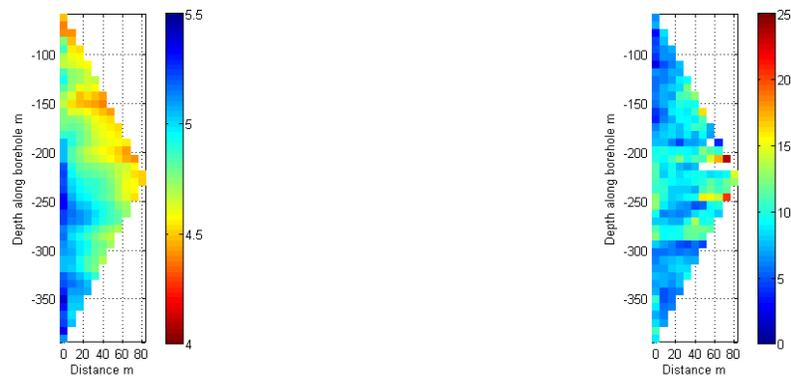
**Figure 3.3:** Apparent resistivity (left) and chargeability (right) pseudo-sections along borehole W128 (Schlumberger array). Resistivity is in  $\log_{10}(\Omega m)$ . Chargeability is in  $mV/V$ . Electrode spacing is 8m
