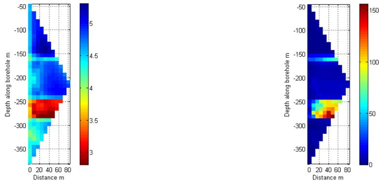
Figure C.4: Apparent resistivity in  $\log_{10}(\Omega m)$ (left), chargeability in  $mV/V$  (right) pseudo-sections of NRS170143
