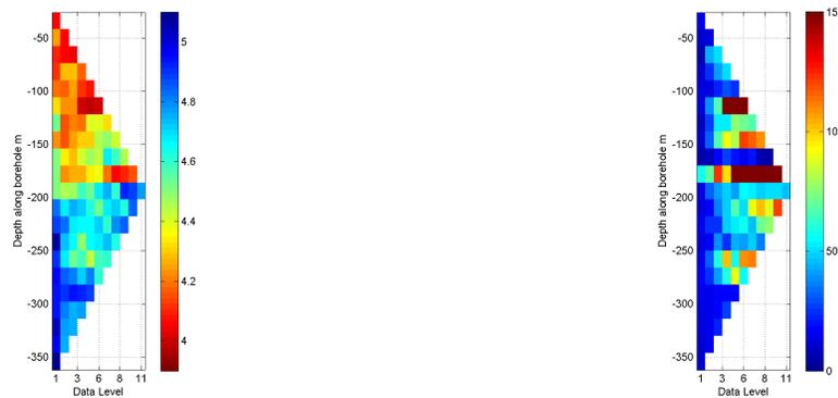
**Figure 4.10:** Apparent resistivity (left) and chargeability (right) pseudo-section along BR3 (Schlumberger array). Resistivity is in  $\log_{10}(\Omega m)$ . Chargeability is in  $mV/V$ . Electrode spacing is 16m
