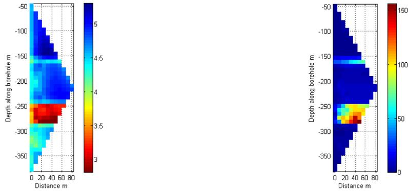
**Figure 3.9:** Apparent resistivity (left) and chargeability (right) pseudo-sections along borehole NRS170143 (Schlumberger array). Resistivity is in  $\log_{10}(\Omega m)$ . Chargeability is in  $mV/V$ . Electrode spacing is 8m
