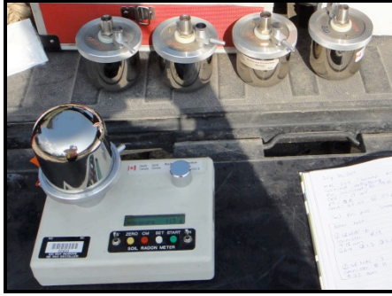
Figure 9: Photograph of ionization chambers and the electrometer used to measure Rn in soil gas.
