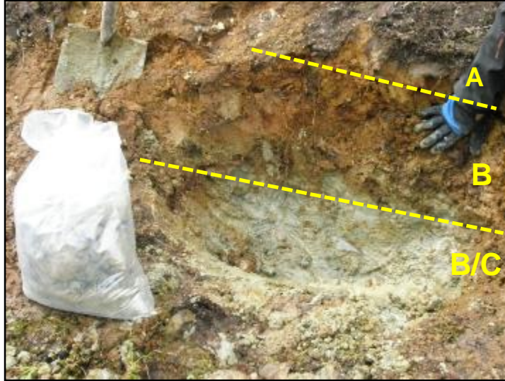
Figure 6: Soil horizons showing the transition from the weathered upper B horizon to the grey/green lower B/upper C horizon.
