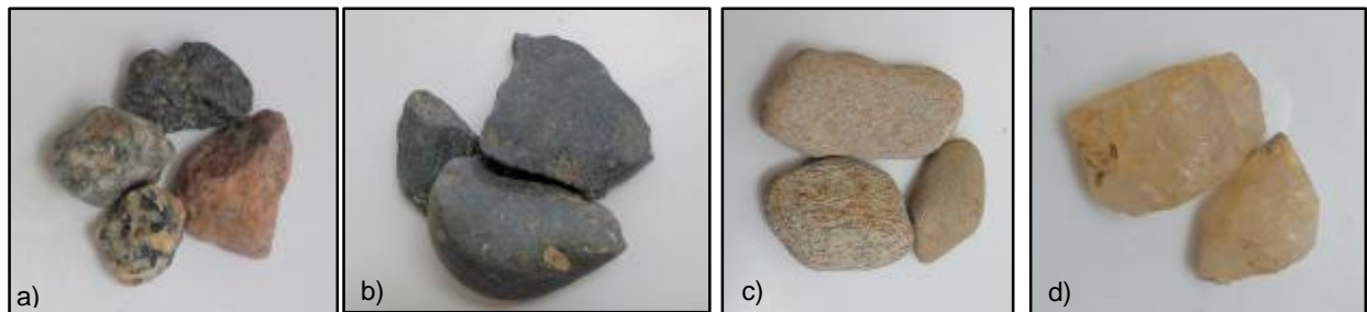
Figure 21: Clast sorting categories: a) Igneous, b) Metasediments, c) Mica-rich Metasediments, d) Quartz, and Miscellaneous (not shown). Metasediments (b and c) combined for pie charts.
