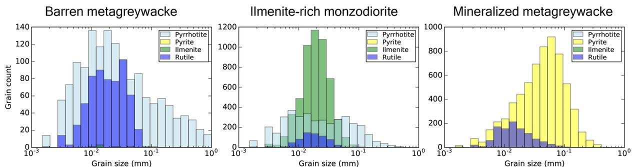
**Figure 4:** Grain size histograms of metallic grains obtained with Mineral Liberation Analysis for the three identified types of SIP spectra. Pyrrhotite replaces pyrite as the main sulfide in barren metagreywacke.
