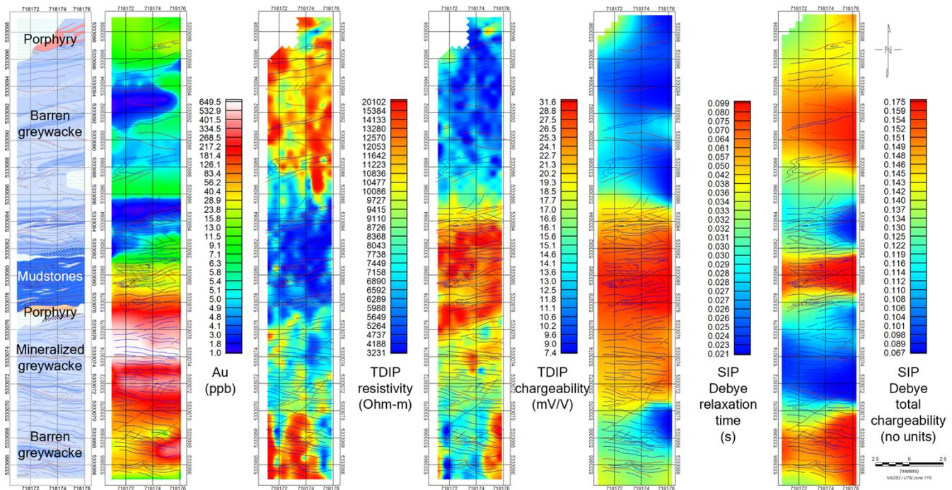
**Figure 5:** From left to right: local geology, gold content (ppb), time-domain resistivity (Ohm-m), time-domain chargeability (mV/V), frequency-domain Debye mean relaxation time (s), and frequency-domain Debye total chargeability (no units) measured on the Bravo zone outcrop.
