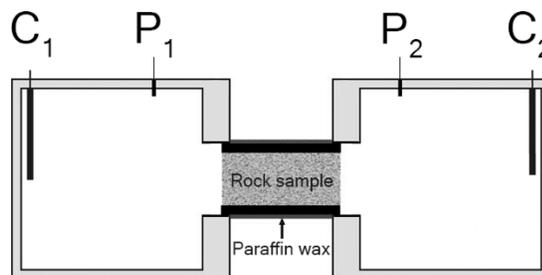
**Figure 2:** Schematic of the sampler holder for SIP measurements. Modified after Zisser et al. (2010).
