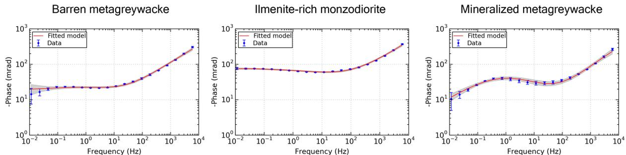
**Figure 3:** Phase shift of the complex resistivity measured on core samples extracted from the BR08-2034 borehole at the Bravo zone outcrop. The fitted Debye decomposition model is drawn in red, with the grey area corresponding to the 95% highest posterior density interval.
